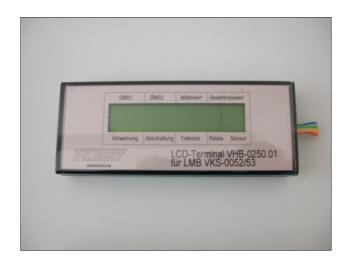
The VHB-0250 is suitable using in new constructions particularly for the first application of the sensors. One can likewise use it for service case use.
