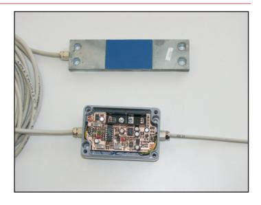
The amplification range can be selected from four steps with a short-circuit bridge for the optimal adaptation of the amplifier. A comparator with a LED is integrated as help for the balance comparison of the force transducer.
