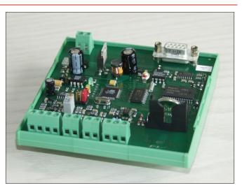
The function of the data logger covers the permanent storage of the four channels in second time. A comparison of the current measurements is permanently carried out with switching thresholds (alarm thresholds) defined before. A transgression or underrun of the thresholds is understood as an event to record in writing and is stored with the date and time.
